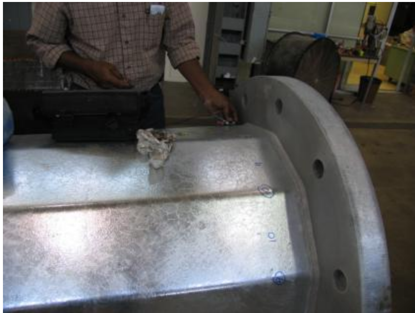
Figure 3.4 Ultrasonic Test Being Performed by a TxDOT Inspector
