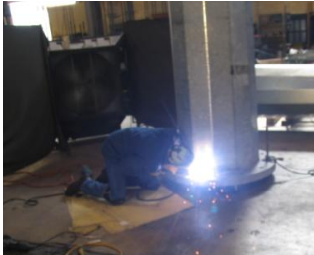
Figure 2.14 SMAW Repair Procedure Performed at Ferguson Lab
