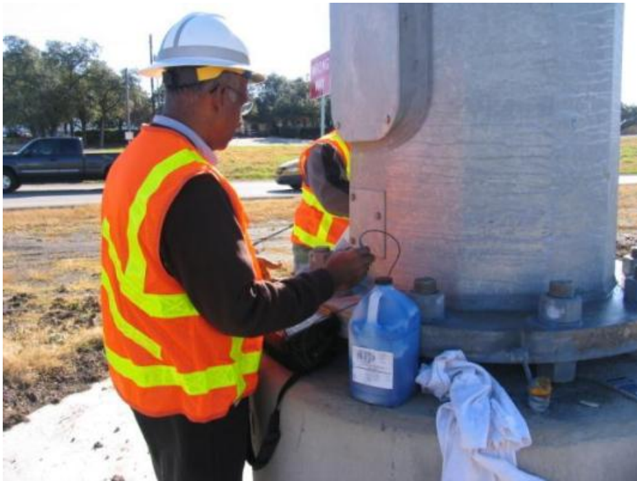
Figure 1.4 Ultrasonic Testing Performed by a TxDOT Inspector
