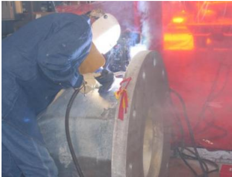
Figure 2.12 FCAW Being Performed at the Ferguson Lab
